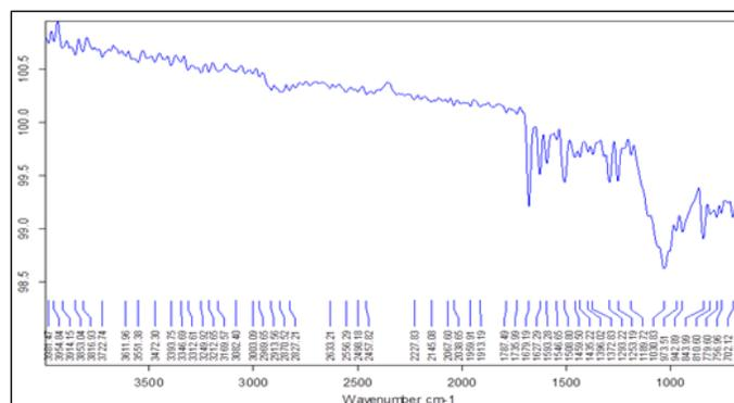
**Figure 4:** FT-IR Spectra of Apixaban Solid dispersion (batch no. APX71).
