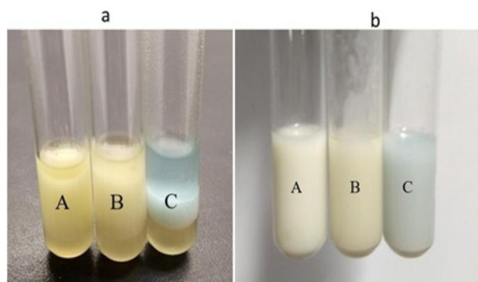
**Figure 4:** (a) Partial emulsification of Hydrocarbons A) Crude oil B) Petrol C) Kerosene using partially purified biosurfactant alone. (b) Complete Emulsification of Hydrocarbons A) Crude oil B) Petrol C) Kerosene using partially purified biosurfactant and pyocyanin. All the analysis were carried out in triplicate.
